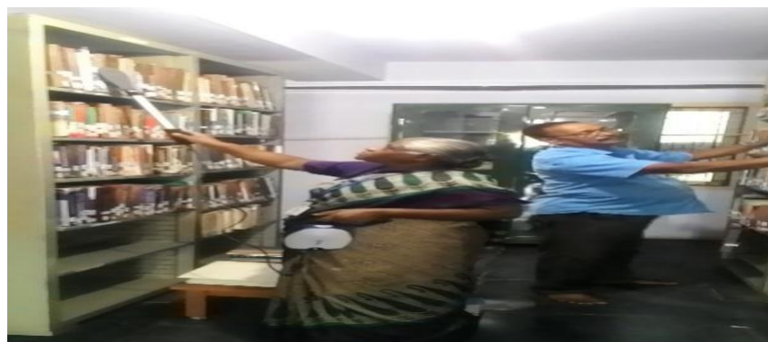
Fig.5 A WIFI inventory control system is used for stock taking ,finds the misplaced books in the book shelf and shelf rectification purpose.
